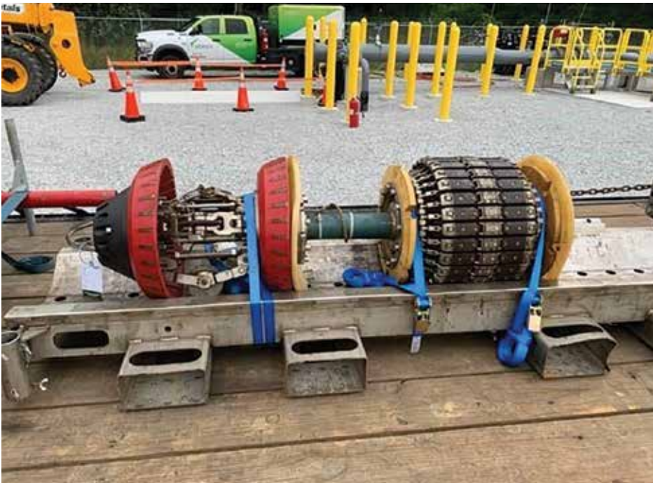
16" ILI magnetic flux leakage tool used to assess metal loss
